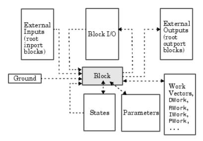
An S-function's mdlInitializeSizes routine sets the sizes of the various signals and vectors. S-function methods called during the simulation loop can determine the sizes and values of the signals.
