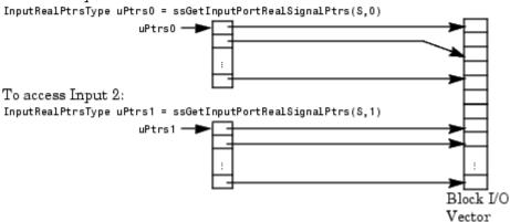
As shown in the previous figure, the input array pointers can point at noncontiguous places in memory.
