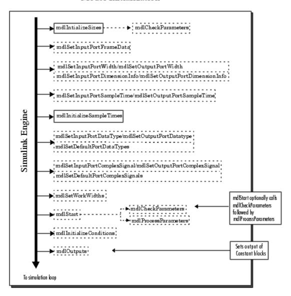
Note The mdlInitializeSizes callback method also runs when you enter the name of a compiled S-function into the S-Function Block Parameters dialog box.
