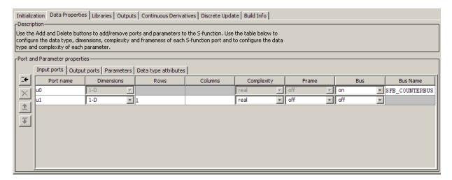
The column of buttons to the left of the panes allows you to add, delete, or reorder ports or parameters, depending on the currently selected pane.
