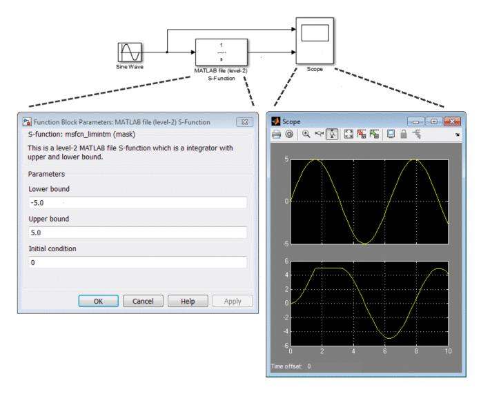
The model  ${\tt msfcndemo\_limintm}$  in this example incorporates the sample S-function  ${\tt msfcn\_limintm.m}$ .
