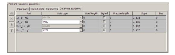
The pane contains a table listing the data type attributes of each of the S-functions ports. You can edit only some of the fields in the table. The other fields are grayed out. Each row corresponds to a port of the target S-function. Each column specifies an attribute of the corresponding port.
