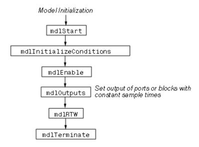
If the S-function resides in a conditionally executed subsystem, it is possible for the generated code to interleave calls to mdlInitializeConditions and md1Start. Consider the following Simulink model sfcndemo enablesub.
