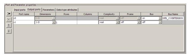
The pane consists of a table that lists the properties of the output ports in the order in which the ports appear on the S-Function block. Each row of the table corresponds to a port. Each entry in the row displays a property of the port as follows.
