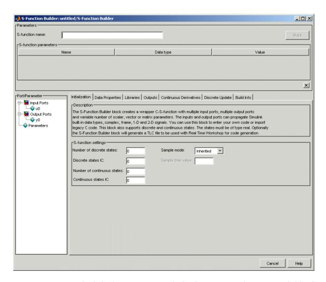
The dialog box contains controls that let you enter information needed for the S-Function Builder block to build an S-function to your specifications. The controls are grouped into panes. See the following sections for information on the panes and the controls that they contain.
