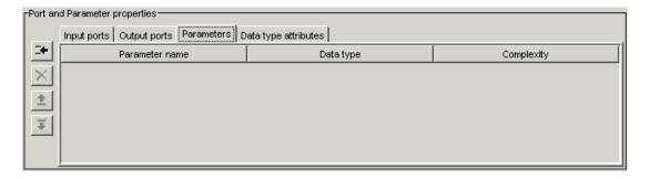
The pane consists of a table that lists the properties of the S-function parameters. Each row of the table corresponds to a parameter. The order in which the parameters appear corresponds to the order in which the user must specify them in the **S-function parameters** field. Each entry in the row displays a property of the parameter as follows.
