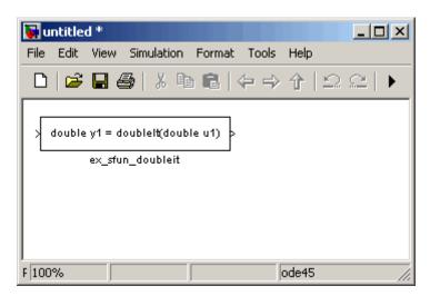
The following Simulink model demonstrates that the C MEX S-function produced by the Legacy Code Tool behaves like the C function doubleIt. In particular, the S-Function block named ex\_sfun\_doubleit returns the value of its floating-point input multiplied by two.
