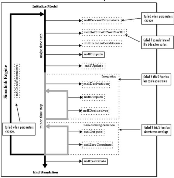
If your model contains multiple S-Function blocks, the engine invokes a particular method for every S-function before proceeding to the next method. For example, the engine calls all the mdlInitializeSizes methods before calling any mdlInitializeSampleTimes methods. The engine uses the block sorted order to determine the order to execute the S-functions. See "What Is Sorted Order?" in *Using Simulink* to learn more about how the engine determines the block sorted order.
