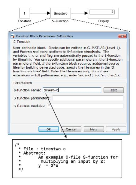
In this example, the model contains an S-Function block that references an instance of the C MEX file for the S-function timestwo.c.
