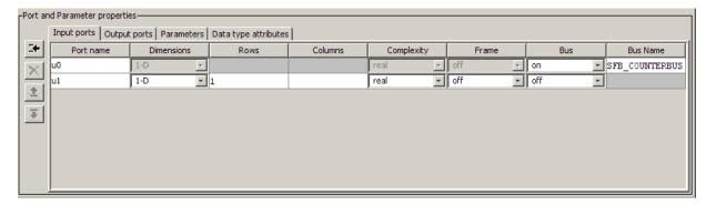
The pane comprises an editable table that lists the properties of the input ports in the order in which the ports appear on the S-Function Builder block. Each row of the table corresponds to a port. Each entry in the row displays a property of the port as follows.
