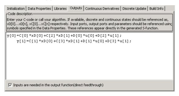
The Outputs pane also selects the Inputs are needed in the output function (direct feedthrough) option since this state-space model has a nonzero D matrix.
