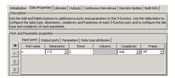
The **Output ports** pane similarly defines the one S-function output port as a 1-D vector with two rows.
