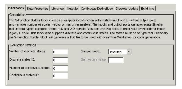
The S-Function Builder uses the information that you enter on this pane to generate the mdlInitializeSizes callback method. The Simulink engine invokes this method during the model initialization phase of the simulation to obtain basic information about the S-function. (See "Simulink Engine Interaction with C S-Functions" on page 4-77 for more information on the model initialization phase.)
